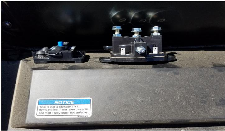
7. Attach the included BLACK ground wire to the GND post on the contactor. Attach the other end to the Accessory Kawasaki Fuse Box ground block.
