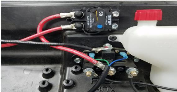
5. Attach the two female spade connectors from the shifter harness to the spades on the contactor. Does not matter what color wire goes to each spade connector.
